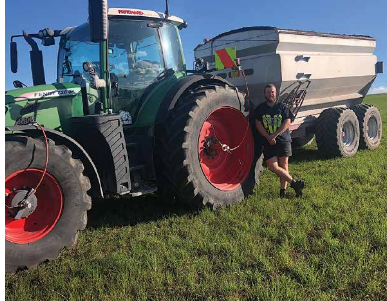
SAM PRITCHARD WITH THE 12-TONNE GILTRAP SPREADER, WHICH HAS HUNGRY BOARDS SO IT CAN CARRY LARGE LOADS OF VERMICAST.
