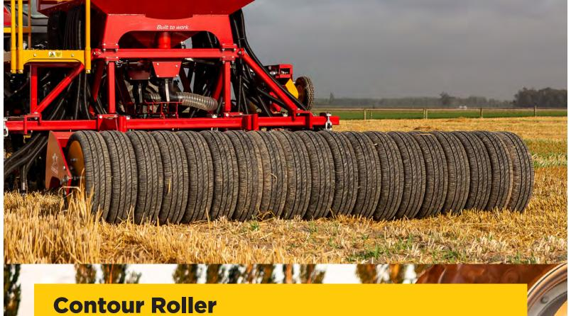
The Contour Tyre Roller has two wheels per independent oscillating assembly for the best ground following ability in closing the slots and ensuring good seed-to-soil contact.
