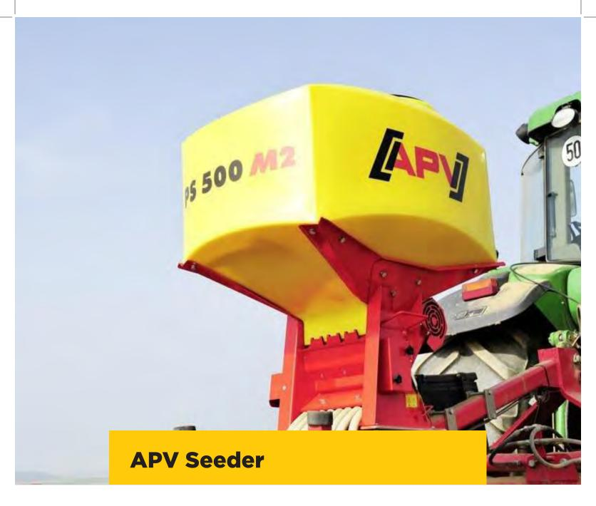
These APV hydraulic or electric air seeding units are suitable as third hoppers on most Duncan drill models. Ideally suited for broadcasting cover crops in the same pass as sowing the main crop.
